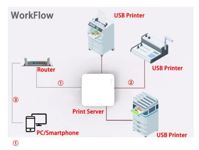
If it's Network USB print server, please connect Router with print server via RJ45 cable; If it's WIFI USB print server, it is ok to connect Router with print server via WiFi direclty; If it is Bluetooth Network USB print server, you prefer to Bluetooth printing, It doesnt need to connect Router with print server.
