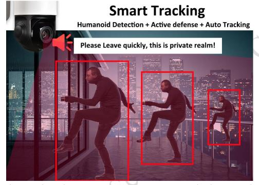
The Network PTZ dome camera supports preset position guard and cruise guard to recognize humanoid automatically. Once the detection is trigged, the security PTZ dome camera automatically turns to the target position, flashing the visible light, and the audio output line drives the live speaker to send out the voice.
