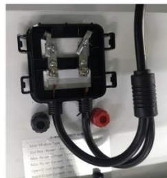
S3: Open the solar power output panel, Red Connector: Positive +, Black: Negative -
